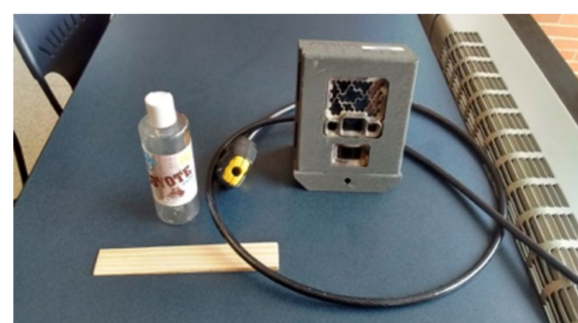
Figure 1. Reconyx Game Camera (HC600 Hyperfire) with security housing, titanium lock, wooden stake, and coyote urine.
